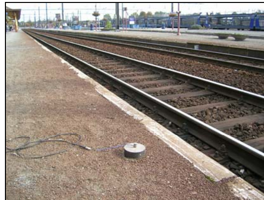
Determination of the dynamic deformations of floors due to rail traffic (railway station Ath)
